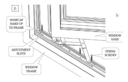
2. FIT THE SASH TO THE FRAME. ENSURE THAT THE NOSE CAPS ARE PUSHED UP TO THE FRAME CORNER AND FIX IN POSITION. ADJUSTMENT IS PROVIDED BY THE ADJUSTMENT SLOTS IF REQUIRED.
