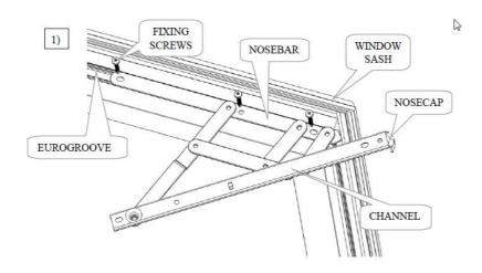
1. PLACE THE FRICTION HINGE NOSE BAR ONTO THE SASH EUROGROOVE AND FIX IN POSITION. THE POSITION WILL DEPEND UPON THE WINDOW PROFILE USED.
